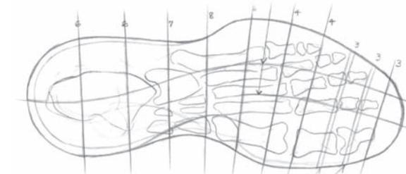
A sole grid pattern was created to match the exact structure of the foot and motion data. The heel is split to mimic the roll through from contact to push off. The big toe is split from the other toes for excellent push off and the reverse grooves in the forefoot allow the smaller toes to grip the earth.
